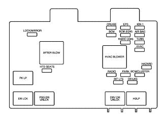
The instrument panel fuse block is located on the passenger's side of the lower console.
